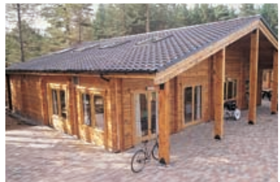
A timber pavilion and information centre. The recessed frontage and the use of all-timber construction creates an attractive and robust building for this rural location.
